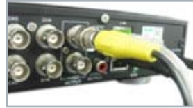
Plug RCA cable to BNC
